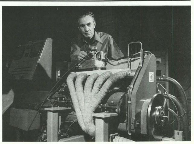
THE MAN AND THE ENGINE — Inventor Harvey Pouliot and variable displacement engine that offers significant fuel economy. Harvey is a member of Sandia Livermore's Combustion Applications Division (8116).
